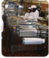
A combined power and communication cable strings together motors on this horizontal form/fill/seal machine, redirecting power away from idle motors to conserve electricity that otherwise would generate heat instead of motion.
